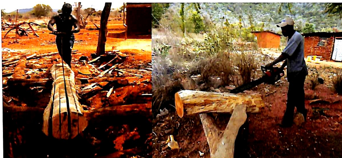
Photograph 6: Melia timber sawing techniques using: Pit saw (left) Power saw (right)
